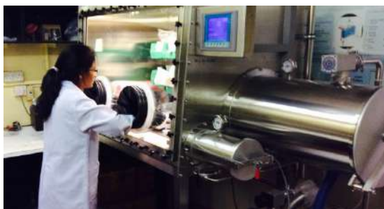
Figure 1: Assembling of rechargeable batteries
