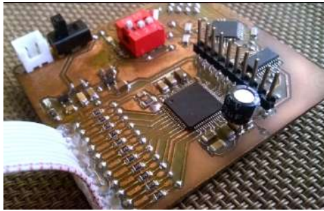
Figure 4: EEG/EMG/EOG Amplifier circuit board constructed in our lab at NIFS
